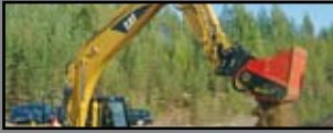
ALLU Bolting grinders Bolting, grinding, mixing, aeration and loading in one operation
